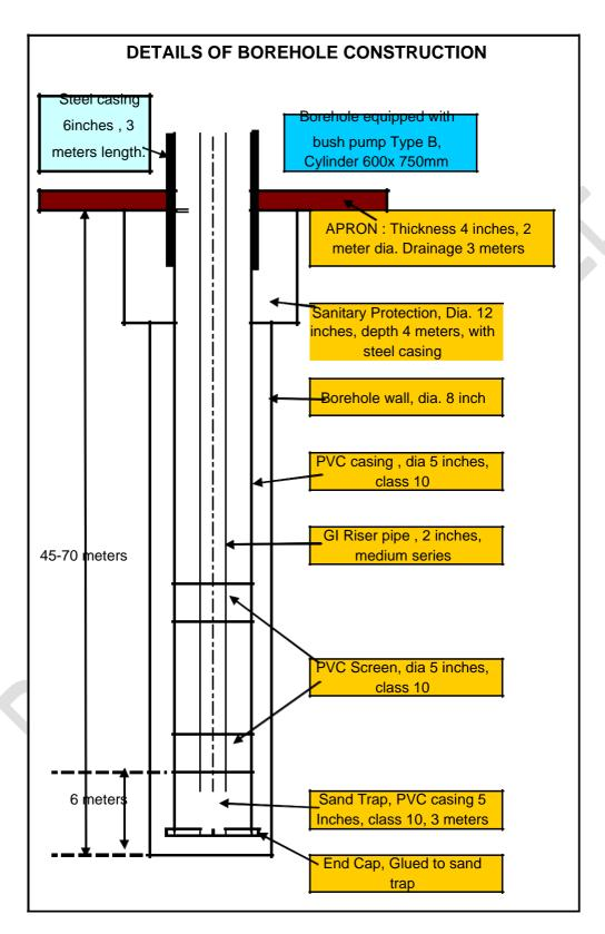
Note: PVC casing & screen Nominal diameters are 6 inches and not 5 inches as shown in the figure.
